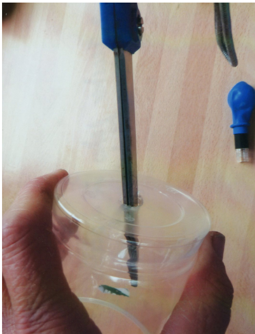
2. Making hole larger for plastic tube
