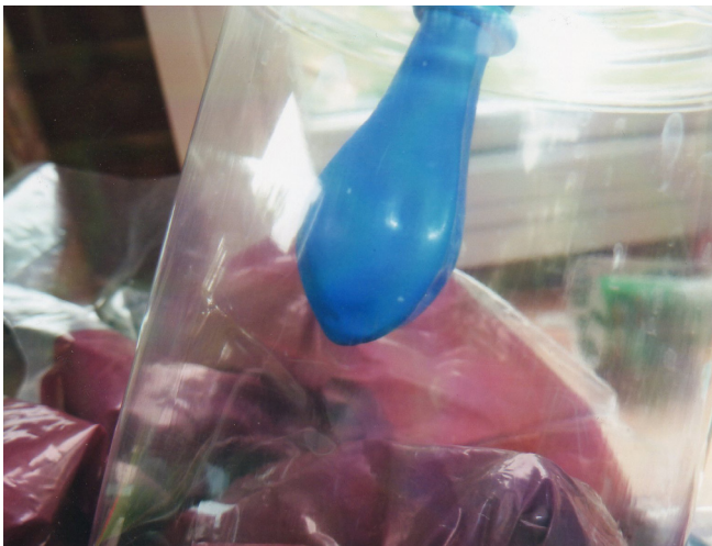
3. Insert tube then attach balloon and lastly thick plastic sheet as diaphragm
